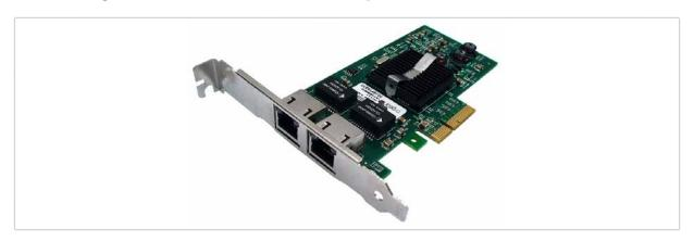
Apply two Gigabit copper server connections in a single PCI Express \* slot.
